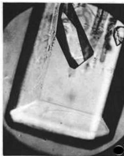
Figure 2. An example of phase transition in a transparent single crystal of p -dichlorobenzene. It is a growth of well-shaped single crystal of the new (higher-temperature) phase within the original single-crystal phase. The transition started from a visible crystal defect at T > T_0 by several degrees. There is no rational crystallographic orientation relationship between the original and new phases
