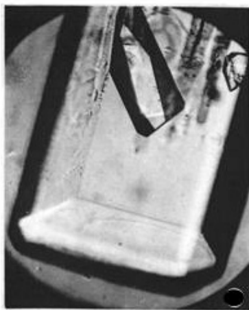
Figure 1. An example of phase transition in a transparent single crystal of p -dichlorobenzene. It is a crystal growth of well-shaped single crystal of the new (higher-temperature) phase within the lower-temperature phase. The transition started from a visible crystal defect at T_n > T_0 by several degrees. There is no rational crystallographic orientation relationship between the initial and new phases
