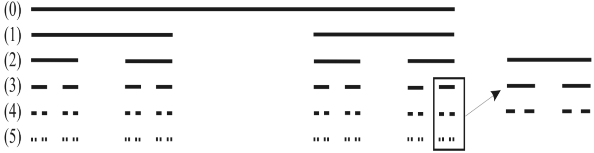
Figure 3. Constructing a pre-Cantor grating of the five order
