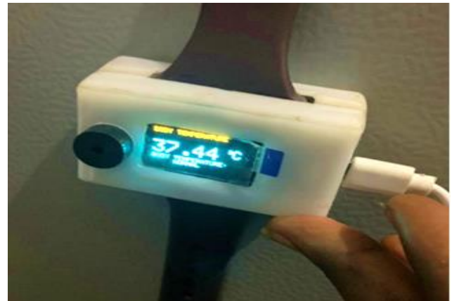
Figure 7. The developed wearable temperature measuring device (WTMD) after packaging
