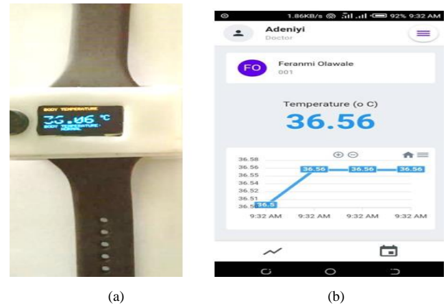
Figure 11. (a) Digital display of temperature on the WTMD and (b) Graph of transmitted temperature displayed on Android mobile app
