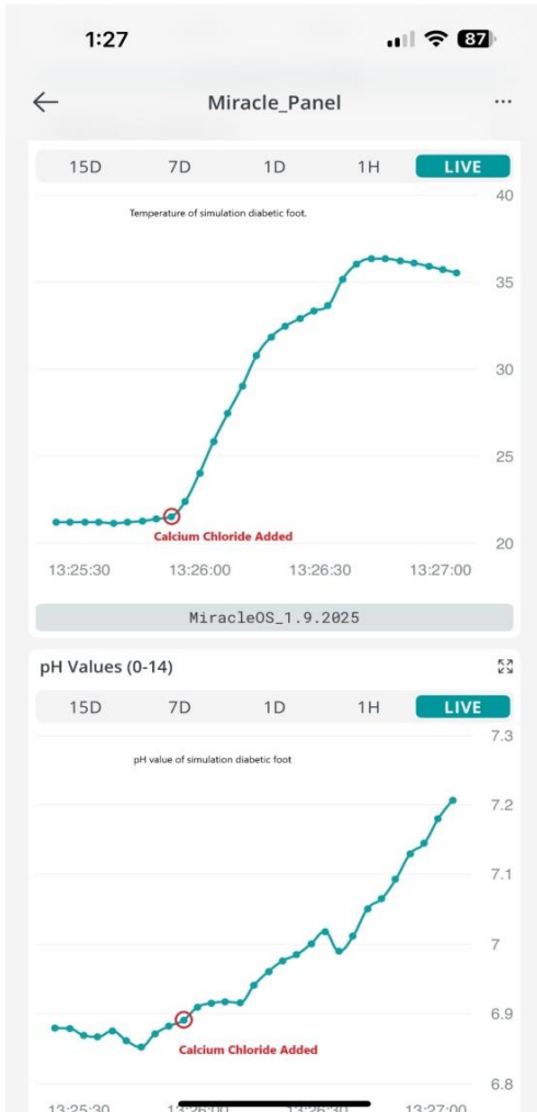
Figure 8. The graph of the values of the temperature (top) and pH (bottom), before and after calcium chloride was added
