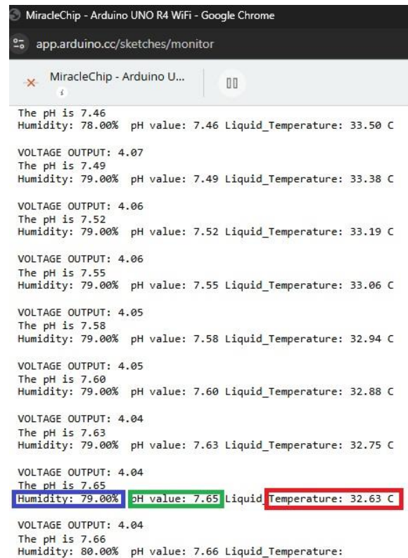
Figure 7. Values of the sensors from the terminal after the addition of calcium chloride
