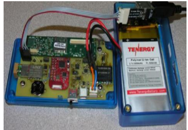
Figure 2. Holster unit containing wireless sensors and batteries
