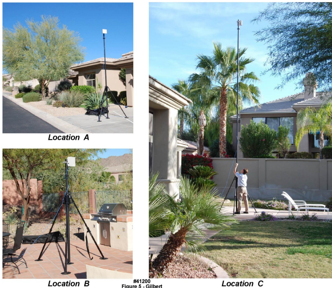
Figure 5. Antenna and mast configuration for the RF transmission of engineering test data from the homes of several volunteers in Scottsdale AZ; receiving base station was located on a building at Mayo Clinic Scottsdale (not pictured)
