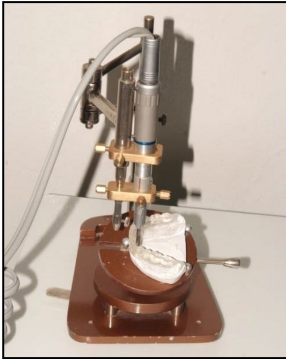
Figure 3. Specially designed copper plate with 2 holes and 2 screws attached to the dental surveyor mandrill
