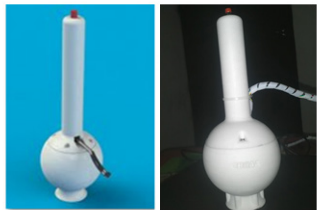
Figure 3. Optoelectronic device for monitoring pupil changes
