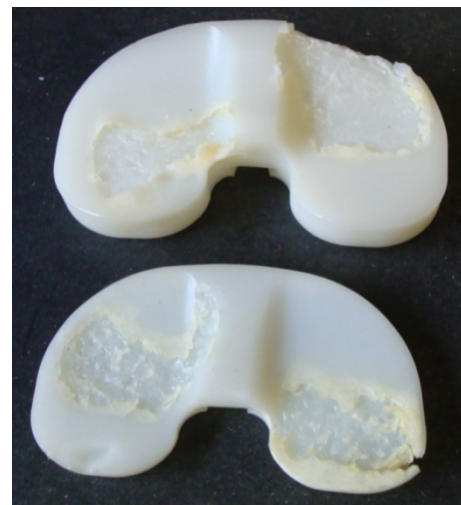
Figure 3. Representative image of a retrieved tibial component from patient with a failed implant device. Note the extensive wear, delamination and cracks.
