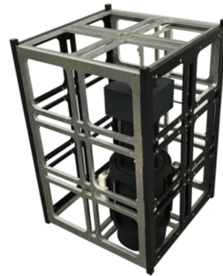
Figure 3. Example of CubeSat structure with removable side panels [20]
