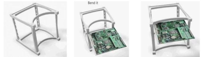
Figure 6. Innovative CubeSat A2 2015 structure [24]
