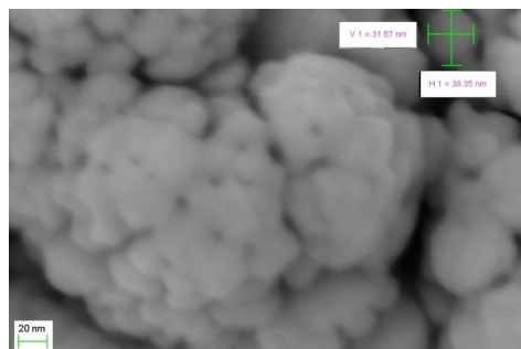
Figure 2. SEM image of nano-Silicalite-1
