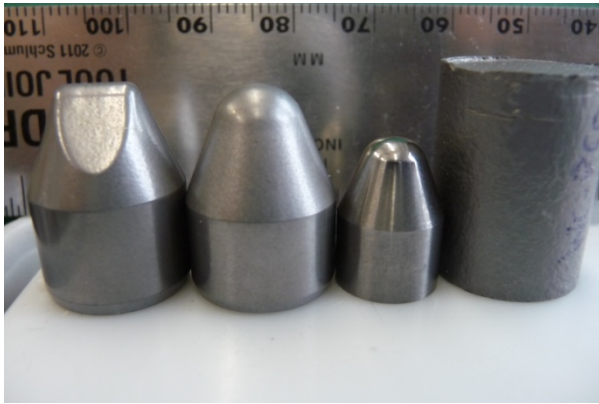
Figure 1. Inserts for tests with the drill hammer and raw cylindrical sample after sintering with the FAST technique
