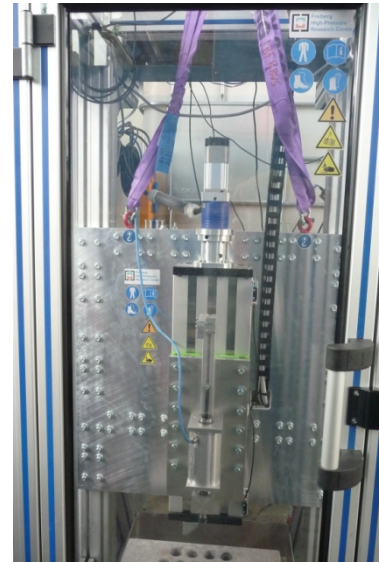
Figure 2. Typical experimental set-up in the small scale drilling test stand
