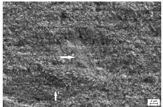
Figure 6. SEM Micrograph from WC- 8Co FAST sample after testing in sandstone
