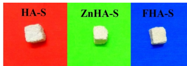
Figure 2. HA-S, ZnHA-S, and FHA-S scaffolds prepared in present work
