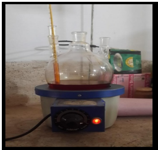
Figure 1. Transesterification of Lard oil
