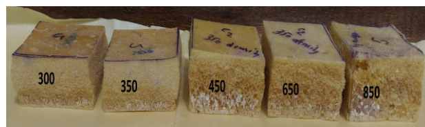
Figure 9. Specimens after Applying Flat Wise Compression Load
