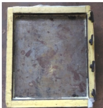
Figure 2. The Mould Used to Fabricate PUF's
