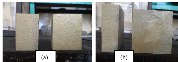
Figure 5. (a) Specimen for Flat Wise Compression (b) Specimen for Edge Wise Compression Test
