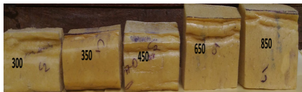
Figure 11. Edge Compressed Specimens
