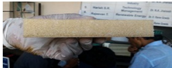
Figure 4. Specimen for Flexural Test
