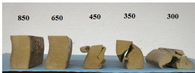
Figure 10. Edge wise compressed specimens
