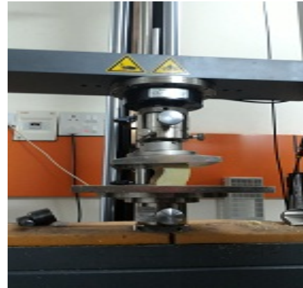
Figure 8. Edgewise Compression Test
