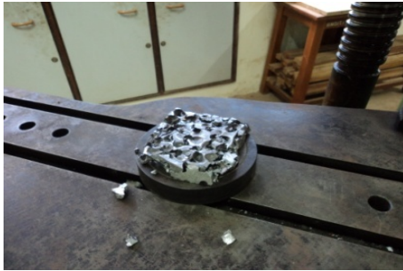
Figure 8. AFSP after compression
