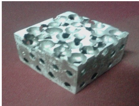
Figure 10. Specimen without face sheets
