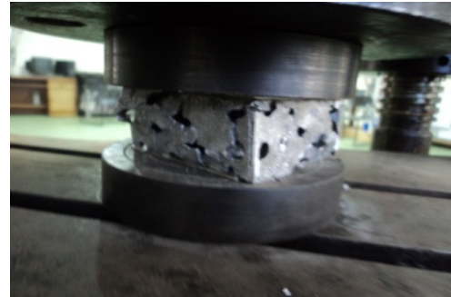
Figure 12. AFSP during compression
