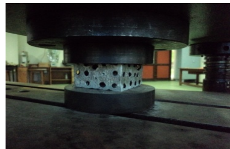
Figure 6. AFSP before compression
