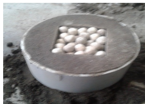
Figure 2. Mould filled with cores
