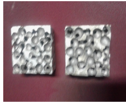
Figure 5. Flatwise Compression Test Specimen
