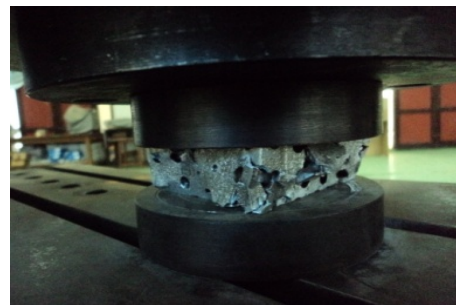
Figure 7. AFSP during compression
