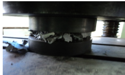
Figure 13. AFSP after compression
