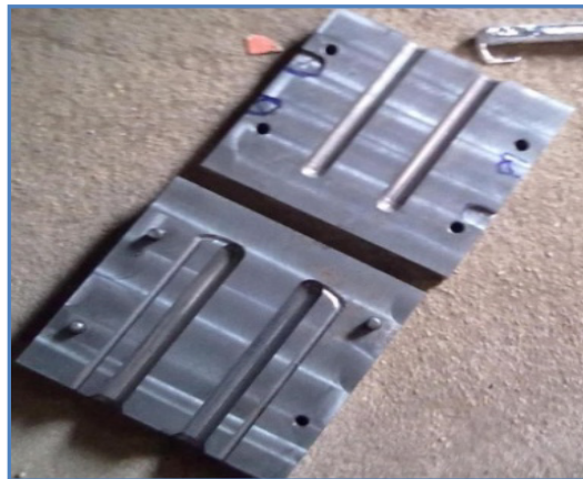
Figure 1. Cast iron die used to prepare the samples
