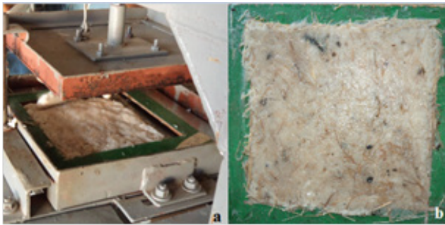
Figure 3. Preparation of biodegradable matrix composites – (a) Mixed constituents ready for compaction (b) Compacted Laminate
