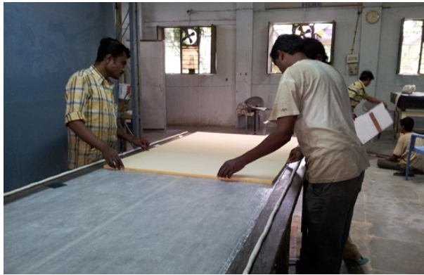
Figure 1. Sandwich panel fabrication
