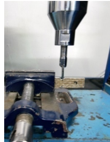
Figure 7. Experimental Setup for Shear Test
