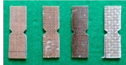
Figure 6. Shear Test Specimen
