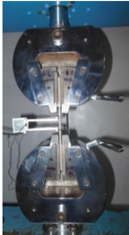
Figure 3. Experimental Setup for Tensile Test
