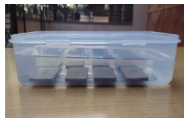
Figure 8. Specimens Immersed in Distilled Water
