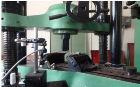
Figure 7. Specimen subjected to Flexural test in computer interfaced UTM with deflectometer set up
