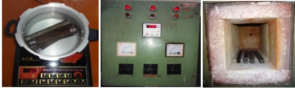
Figure 6. Specimens subjected to hot boiling and kept in Furnace
