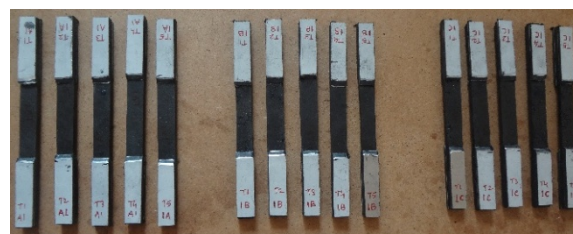
Figure 2. Photograph of tensile test specimen
