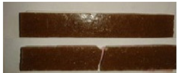
Figure 5. Impact test specimen before and after failure
