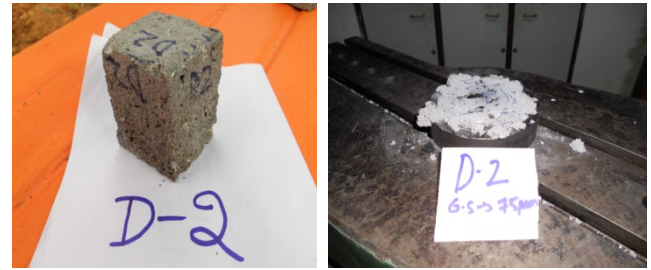
Figure 2. Compression test specimen and specimen after compression
