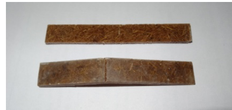
Figure 6. Specimen before and after Flexural testing
