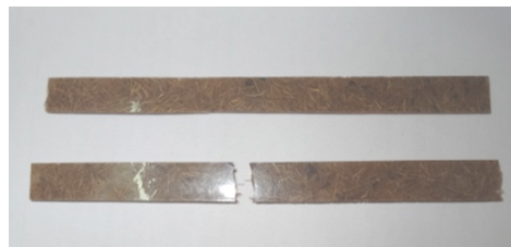
Figure 3. Specimen before and after tensile testing
