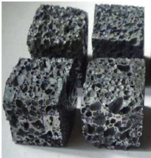
Figure 1. ZA foam cubical sample [18]
