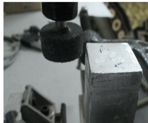
Figure 2. Deburring of rectangular component
