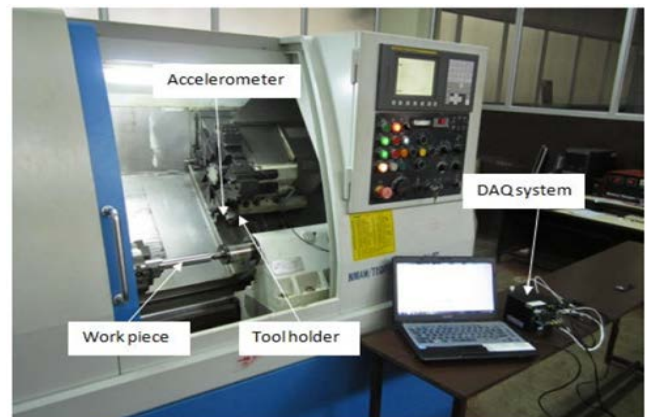
Figure 1. Experimental setup for measurement of cutting vibrations
