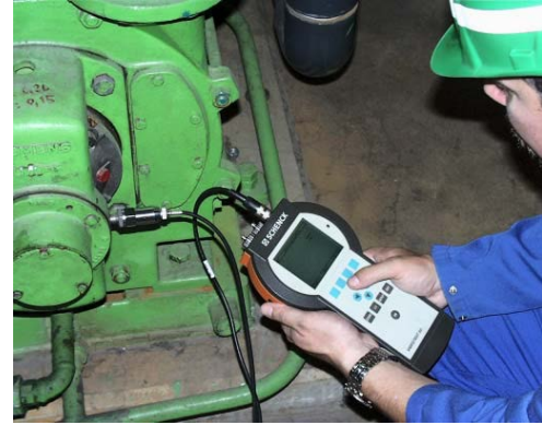
Figure 1. Spindle Vibration Test using Smart Balancer
