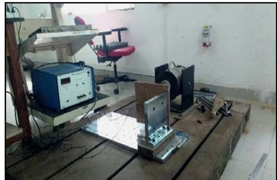
Figure 6. Forced Vibration Test Rig
