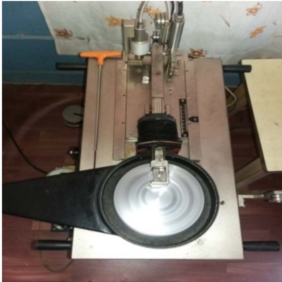
Figure 1. Pin-on-disc setup
