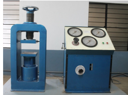
Figure 3. Hydraulic Brick Testing Machine
