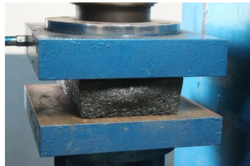
Figure 4. Testing of LDPE/Rubber Composite Brick (Sample 3)
