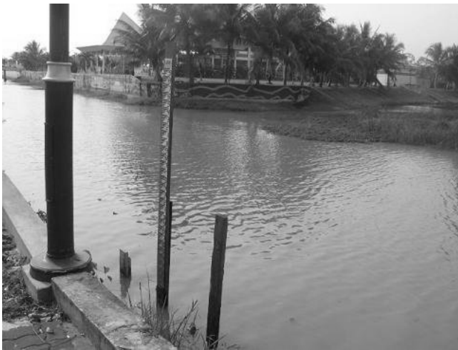
Figure 2. Stick gauge at river station (Source: Department of Irrigation and Drainage Malaysia, 2014)
