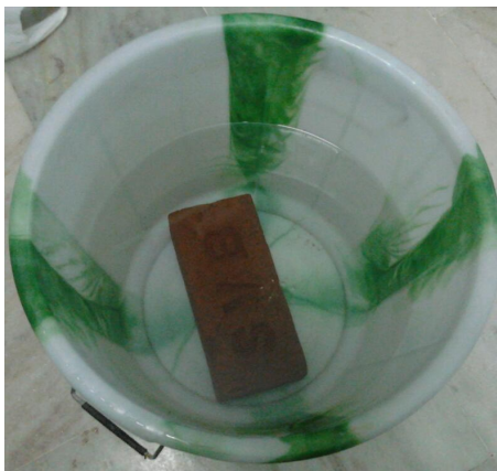
Figure 26. Conventional Bricks Immersed in Water
