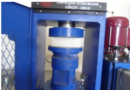
Figure 21. Foam in Compression Test
