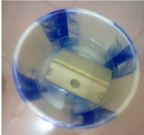
Figure 25. Green Energy Bricks Immersed in Water
