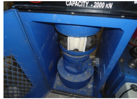
Figure 22. Brick in Compression Test
