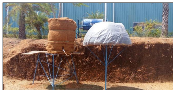
Figure 5. Set-up with blackened collector and insulator with transparent cover
