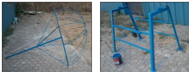
Figure 2. Fabricated dome structure and stand for water storage
