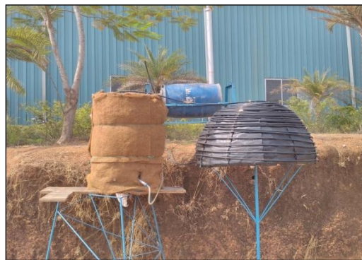
Figure 4. Setup with insulator and collector but without transparent cover
