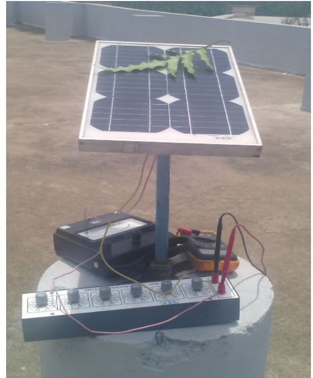
Figure 2. Solar panel under non uniform shading
